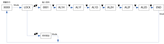
Figure 5-5 Switch point setting flow chart
