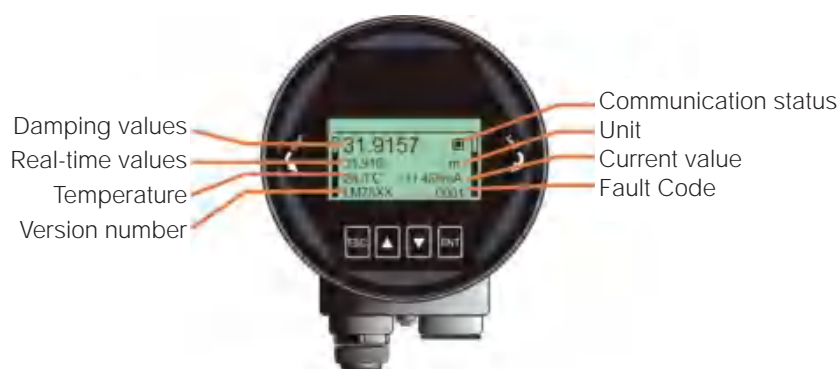
Figure 6-1 Schematic diagram of the running measurement interface
