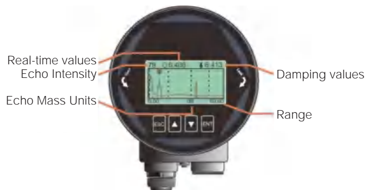
Figure 6-3 Echo curve interface shows the schematic diagram of the TVT curve
